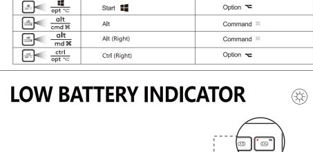
Flashing Red light indicates when the battery is below 10%.
