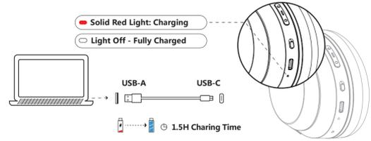
Flashing red light indicates when the battery is below 25%.
